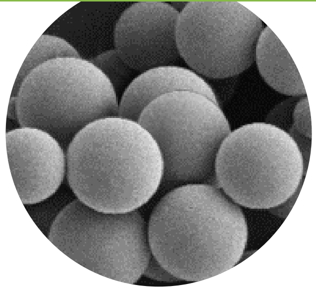
Figure 1: Scanning electron microscopy picture of EmboCept® S DSM 50 µm microspheres
